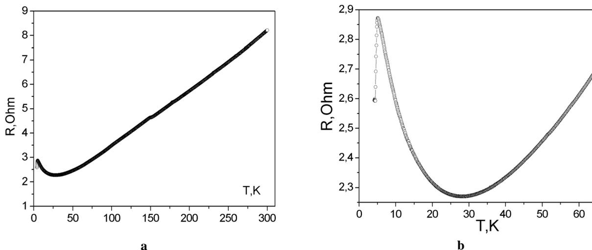
**Fig.1.** Temperature dependence of resistance for n-type Bi<sub>2</sub>Se<sub>3</sub> whiskers with Pd doping concentration of  $1 \times 10^{19} \text{ cm}^{-3}$  in temperature range: a) 4.2 - 300 K; b) 4.2 - 65 K.
